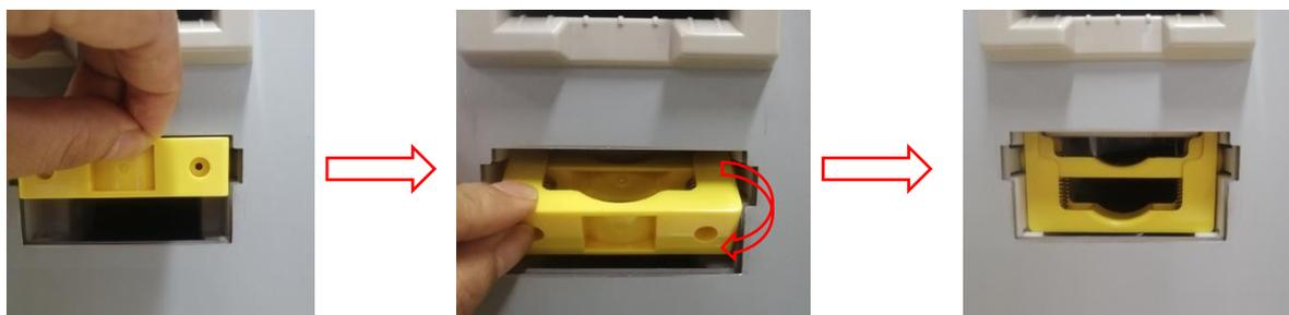
After above steps are completed, then close the upper door to complete the installation of the cleaning module (bottom).
