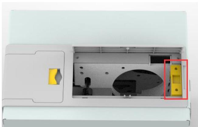
**i** The function of the cleaning roller is to absorb the dust and foreign matter entering the card roller, indirectly stick to the dust on the card surface to improve the printing effect.
