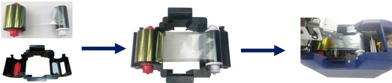
1. Open the upper cover, take out the ribbon cartridge, install the ribbon into the cartridge according to the color direction.
