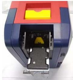
2. Place the card into the input hopper, then add the weight module.
