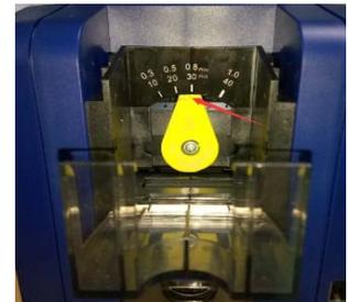
3. Support 0.3mm to 1.0mm thickness cards. Factory preset thickness is 0.8mm.
